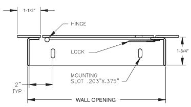
Innovative cost effective access door. 16 ga. return frame and uniweld construction allows for an aesthetically pleasing appearance and square fit in all wall and ceiling applications. The frame is laser cut from one sheet of steel for visual aesthetics.
