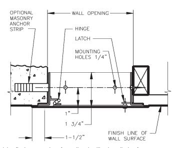
This precision-flush access door for wall and ceiling installation far surpasses other doors because its surround trim is welded on all four sides to the return frame providing strength and rigidity. The frame is laser cut from one sheet of steel for visual aesthetics.
